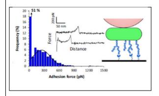
Illustration of single cell force spectroscopy (SCFS) assay in microbiology. The illustration is taken from a review paper (Dufrêne, Trends in Microbiology June 2015, Vol. 23, No. 6) and illustrates the approach used in the study "Single-cell force spectroscopy of probiotic bacteria" (Beaussart, A. *et al.* (2013) Biophys. J. 104, 1886–1892) were carbohydrate interactions of probiotic bacteria were quantified using AFM.
