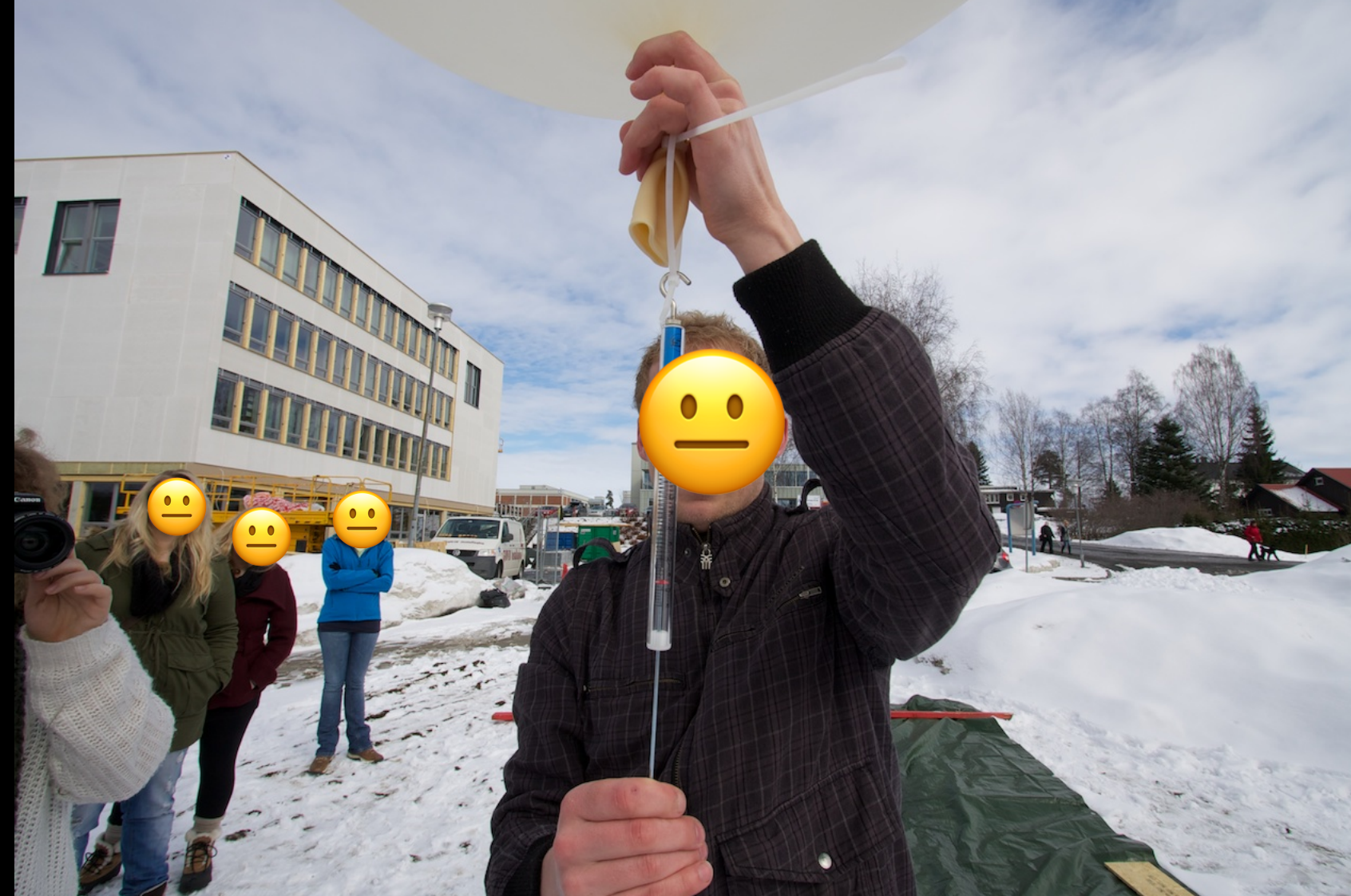
Student measuring the lifting force of the weather balloon using a newton meter
