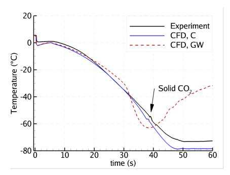
Depressurization of a 200 m tube. Temperature is plotted against time for the position 195 m from the outlet. Experimental data compared to our CFD calculations with two different in-tube heat-transfer models. Notice that only one of the calculations predicts the formation of solid  $CO_2$ .
