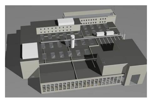
Sketch of the 60 m long depressurization tube on the roof of the Thermal Engineering Laboratories at Gløshaugen.
