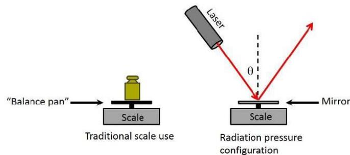
Figure 1. Schematic working principle of a scale configured to be used to measure radiation pressure. Illustration taken from [1].
