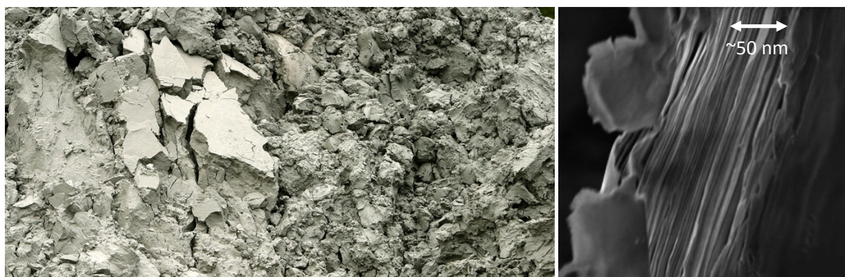
Figure 1 The left panel above is from a natural clay deposit, and it illustrates on a macroscopic scale that clays are anisotropic materials. The right panel is an electron microscope image of vermiculite clay demonstrating its lamellar structure on the nano-scale, reminiscent of graphene, which is one of the main characteristics of clay minerals.
